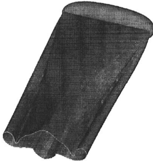
Figure 10. Flow past a stationary rectangular wing at Re = 1000 : iso-surface of streamwise component of velocity corresponding to 97.5% of freestream value
